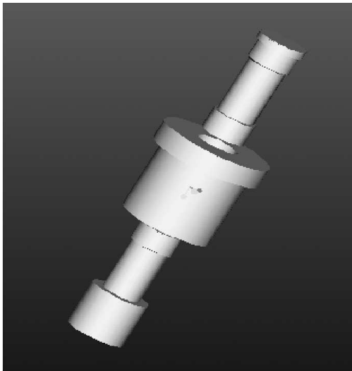
Figure 6. Ceramic Compaction Die Set.
